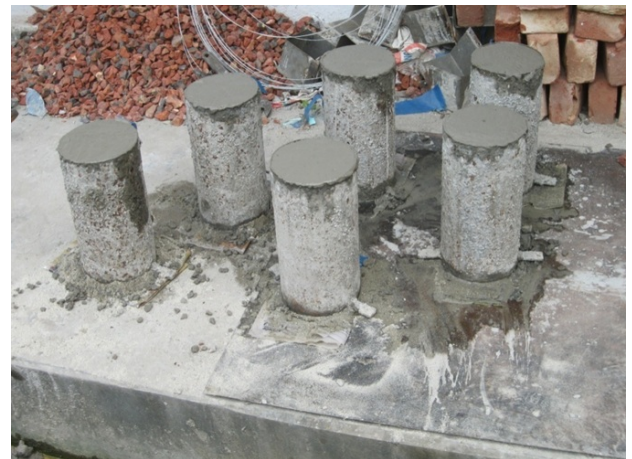
Fig.1: Casting of concrete cylinder
