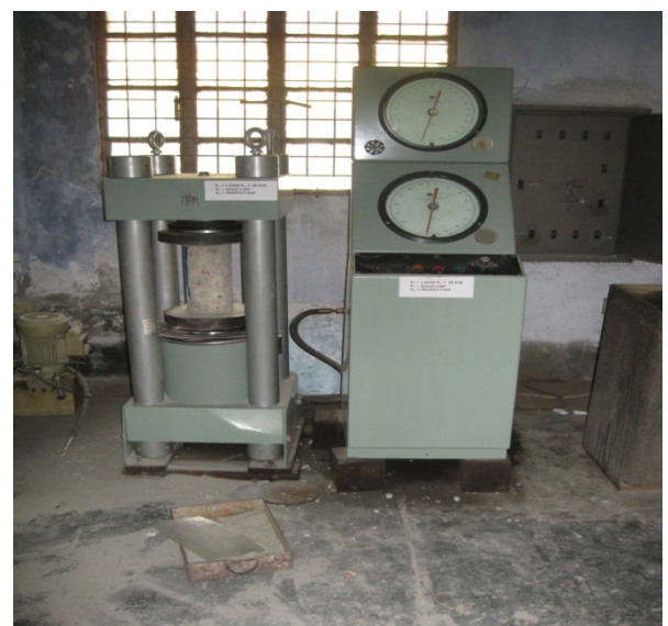
Fig.2: Placing of the specimen in universal testing machine
